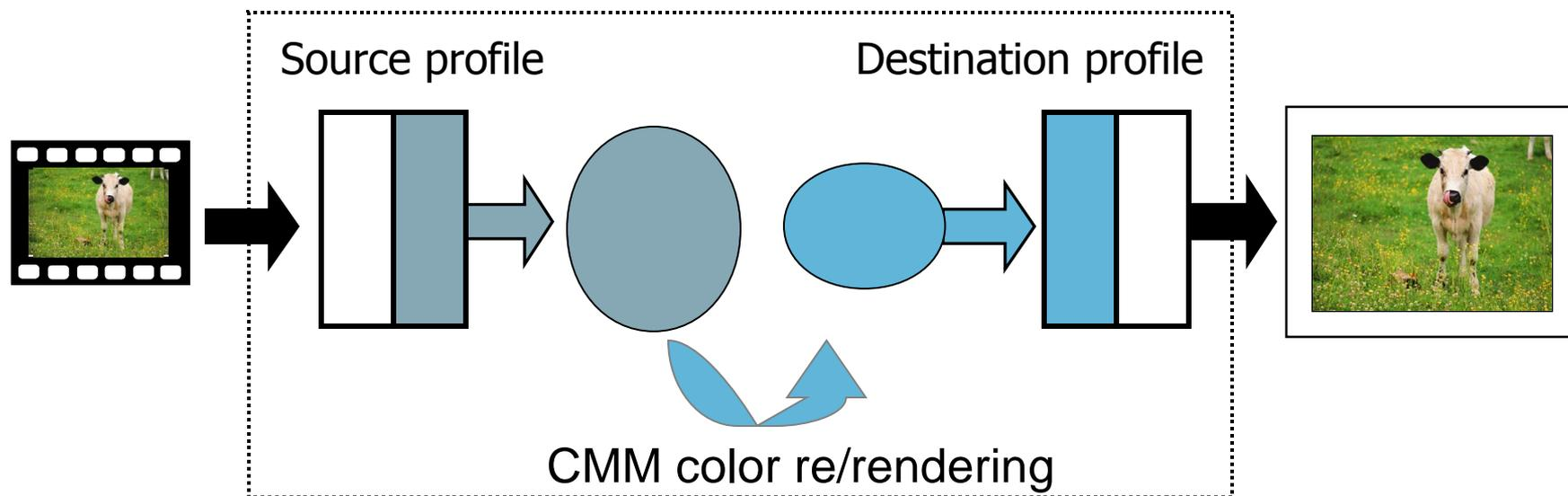
CMM algorithms color re-render source image colorimetry to be appropriate for actual output medium
